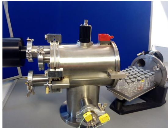
35 vial dryer enabled with dew point sensor , laser absorption , and THz spectroscopy for vapour pressure and TVIS for in-vial behaviour
