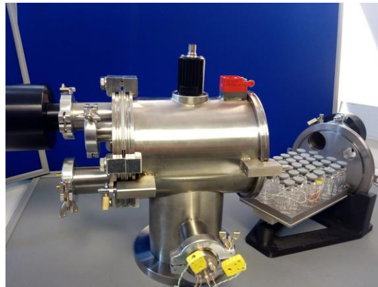
35 vial dryer enabled with dew point sensor , laser absorption , and THz spectroscopy for vapour pressure and TVIS for in-vial behaviour
