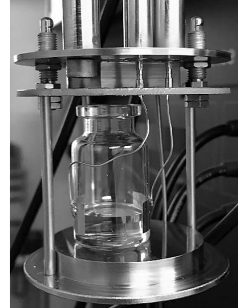
TVIS vial on cradle To be placed in the cryostat of Novocontrol BDS
