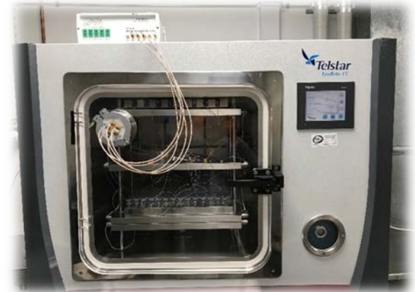
TVIS system connected on Lab Scale Freeze Dryer LyoBeta15, NIBSC, UK
