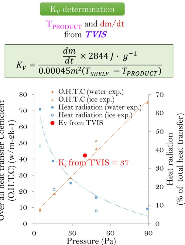
Figure 2.  $K_V$  values for 10 mL tubing vials (Brülls et al. 2002)
