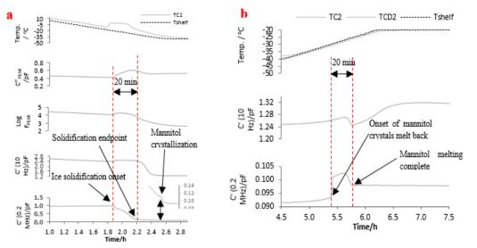
**Fig.1** a) Shows how C"<sub>PEAK</sub>, Log F<sub>PEAK</sub> and Temperature change with time; events that occur with time. b) Demonstrates C"<sub>PEAK</sub> response to the melting mannitol crystals during re-heating period.
