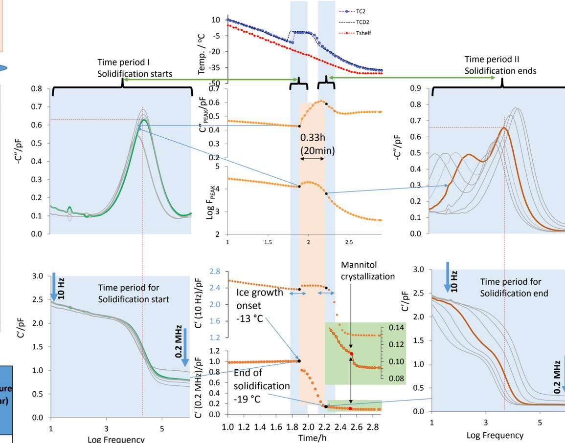
Fig.3  $\log F_{PEAK}$  and  $C''_{PEAK}$  with respect to time depict the events that happened 6 min before and after ice growth onset and during the solidification end point. Spectra around the two major events in the freezing process could assist for more understanding of the happenings during freezing process. In addition, capacitance spectra at lower frequency (10 Hz) and higher frequency (0.2 MHz) show the temperature dependence in the lower frequencies.
