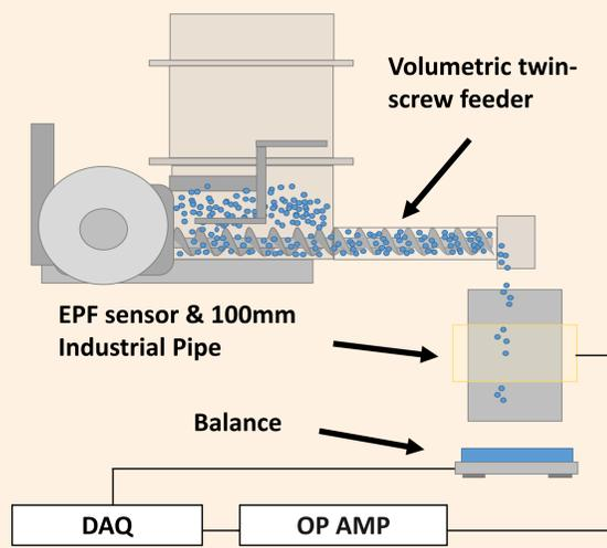
Fig. 3. Schematic of screw feeder and EPF sensor setup.
