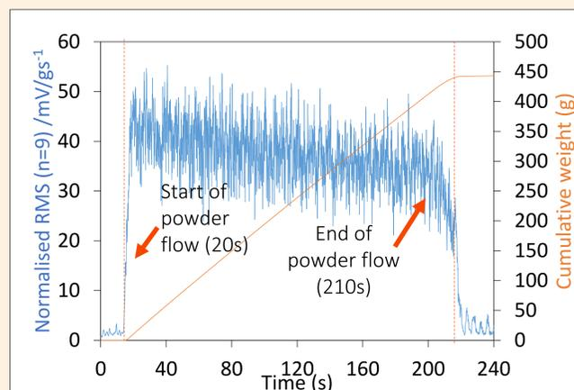
Fig. 4. Normalised RMS and cumulative weight of Avicel PH102 "as received", conveyed at 100rpm through a twin-screw feeder, as a function of time.
