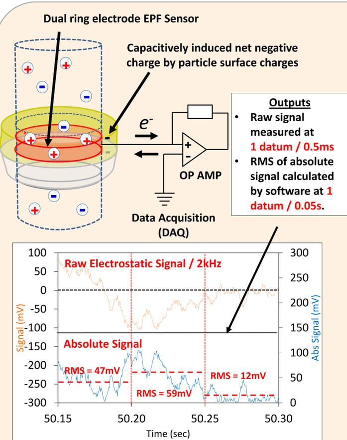
Fig. 2. EPF sensor measurement principle and signal outputs.
