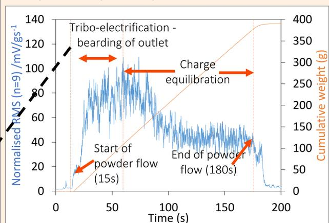
Fig. 5. Normalised RMS and cumulative weight of dried Avicel PH102, conveyed at 100rpm through a twin-screw feeder, as a function of time.
