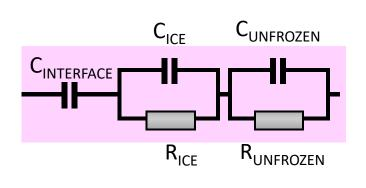
A layers of unfrozen fraction between the ice crystals have dielectric constants and a conductivities which are reflected in  $C_{\rm UNFROZEN}$  and  $R_{\rm UNFROZEN}$ , respectively. The latter is strongly dependent on mobile charge carriers and hence very sensitive to the viscosity (temperature and water content) of the unfrozen fraction .
