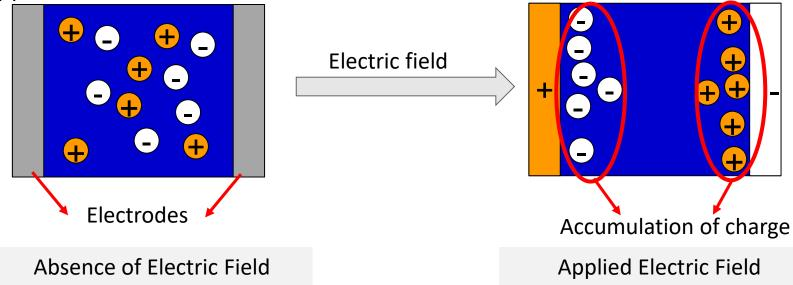
This phenomenon occurs when an electric field is applied to a glass vial (a dielectric material) containing a liquid and/or solid (a dielectric material with some conductivity).
