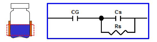
$C_G$  is the capacitance of the glass-solution interface,  $C_S$  and  $R_S$  are the capacitance and resistance of the solution
