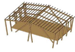
Adding elevated floor level to prevent flooding
