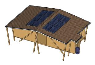
Using solar panels as source of renewable energy and storm water harvesting using roof gutter and water tank for WC usage
